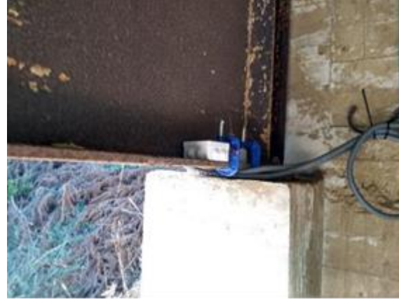
Accelerometer with built-in battery, installed on a steel girder support
