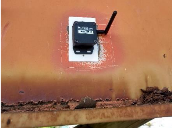
Wireless accelerometer installed on a steel girder
