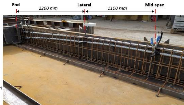
Fig. 2 Lateral view of the half girder scaled by S_L = 5 (a); mid-span cross section (b) and end cross section
