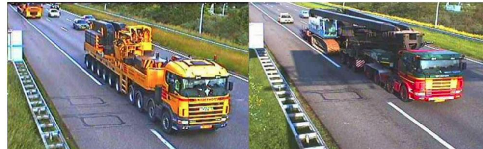
Fig. 1. L: Crane with 10 Axles and Total Weight of 1100 kN, R: Low-loader with 12 Axle and Total Weight of 1650 kN
