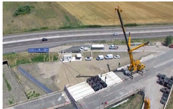
Fig. 1. L: Crane with 10 Axles and Total Weight of 1100 kN, R: Low-loader with 12 Axle and Total Weight of 1650 kN
